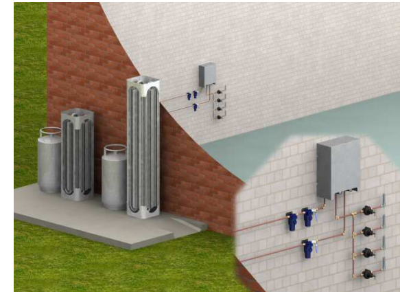
Typical Gas Installation showing the BSL Gas mixer after the liquid gas supply system
